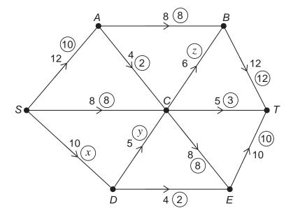
The uncircled numbers on each arc represent the capacity of each pipe in m<sup>3</sup> s<sup>-1</sup>
